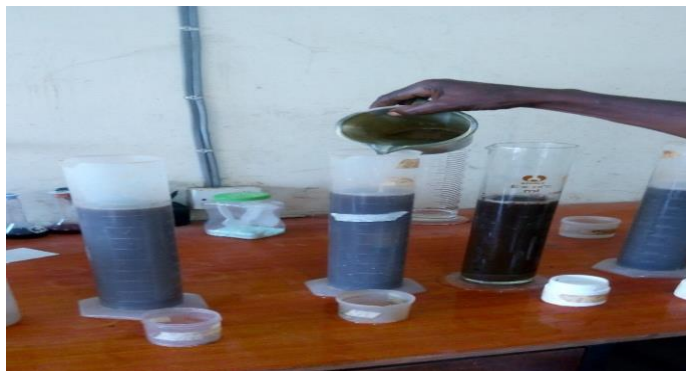
Plate 1. Sedimentation Hydrometer Experiment for Soil Particle Size Determination
