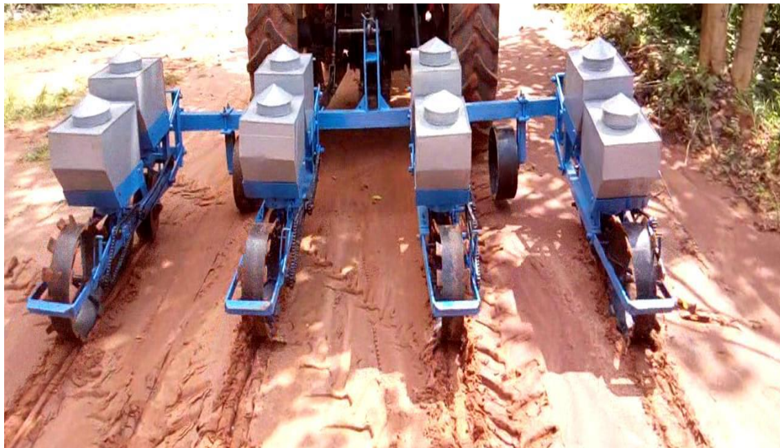
Plate 1. Picture of four-row tractor drawn multi-seed planter
