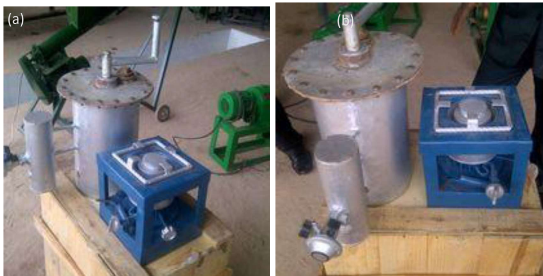
Figure 1 (a) and (b): The fabricated digester and the dual stove
