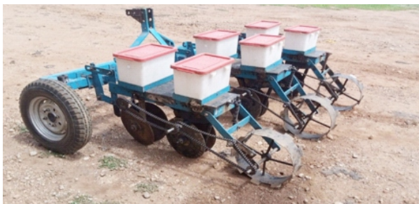
Fig. 3. The fabricated three row tractor drawn multi-seed planter with fertilizer applicator
